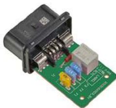
1 Relay, 3 Fast-Blow Fuses, Supporting Electronics 200316-1103 Application Example: Urea Module
