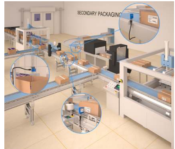
Contrinex C3 Sensors in Secondary Packaging Station
